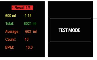
The test mode allows you to immediately check the measurements of the manual ventilator and learn how to use the instrument.
